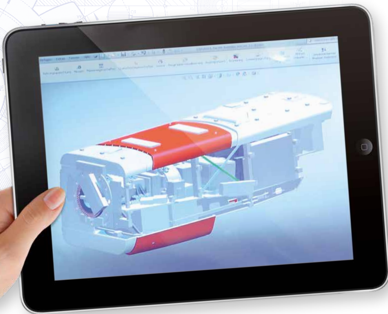
► Nacelle and machine train for the eno 114 / eno 126 as a 3D animation
